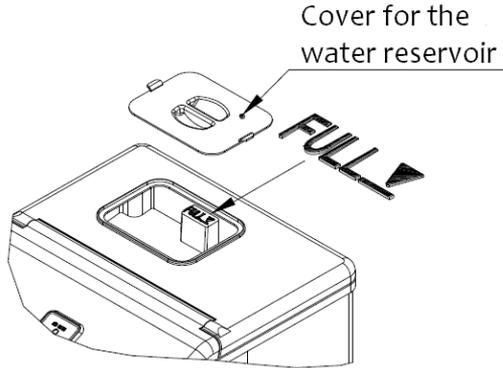
**Please Note:** Do not pour water into the internal water tank located underneath the ice basket. Doing so will affect the ice maker's performance.
